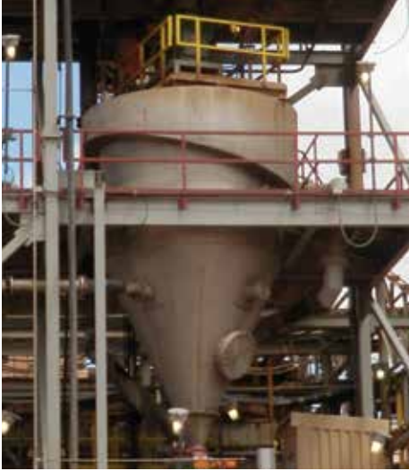
HydroFloat® is an air-assisted density separator for the separation/concentration of minerals that modifies the density of the mineral component. This ten foot (3m) diameter HydroFloat is processing coarse potash.
