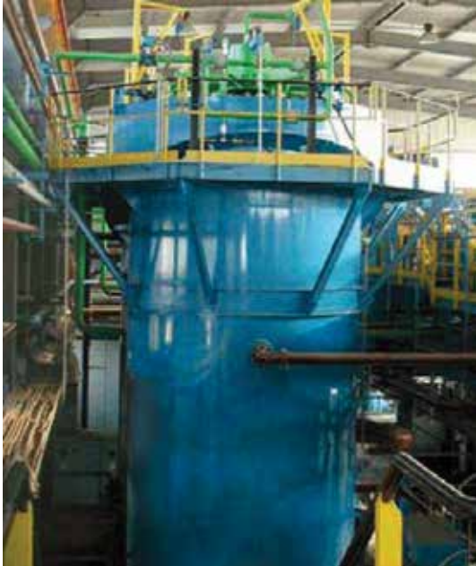
EFD has designed, supplied and commissioned over 800 flotation columns for cleaning, roughing and scavenging duties worldwide.
