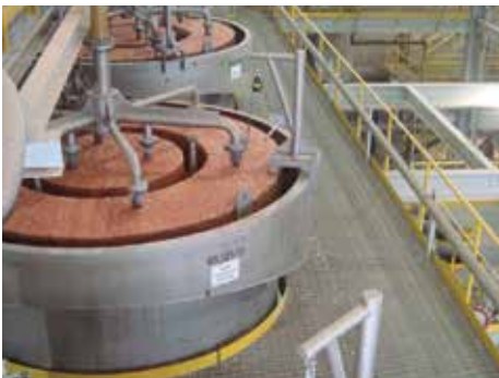
StackCell® offers column-like performance in a substantially smaller footprint than conventional cells. These compact, stackable units offer considerable savings for new installations and are ideal for expanding capacity in an existing plant.
