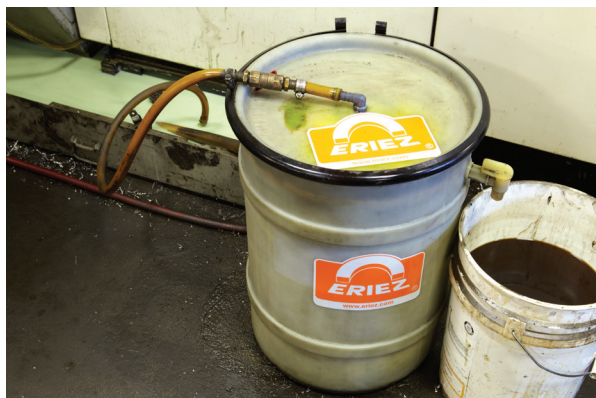
Eriez coalescers are positioned next to a sump to remove tramp oils.
