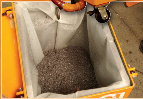
Chips and solids are captured in a large basket.
