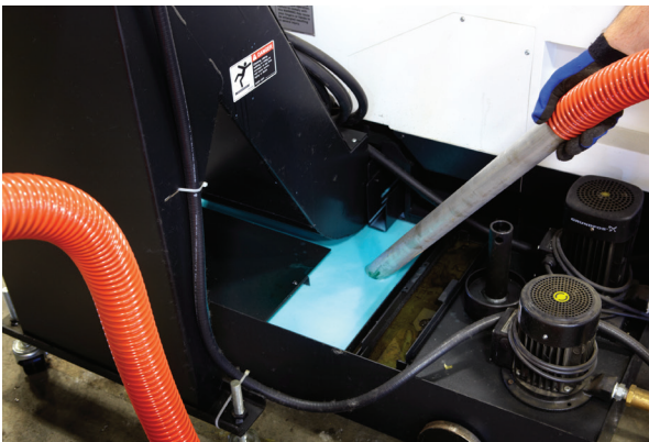
Dirty coolant is vacuumed from the machine's sump.
