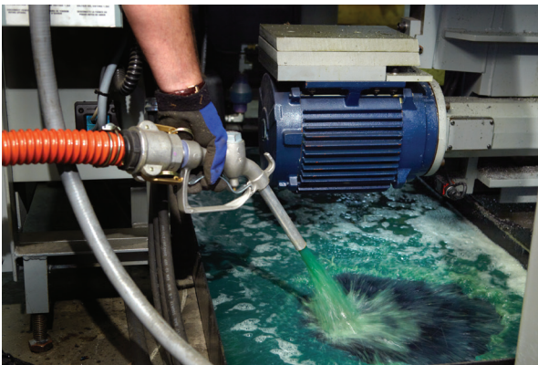
Clean coolant is returned to the machine tool.
